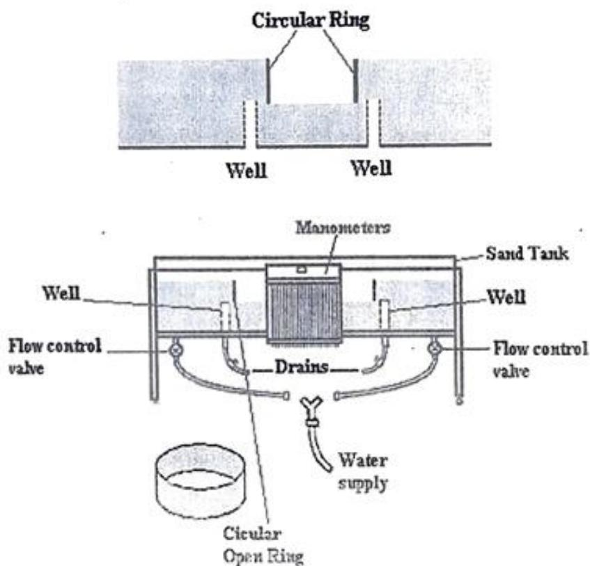
Place the sand tank and smooth the surface to give an even depth of 150 mm.
