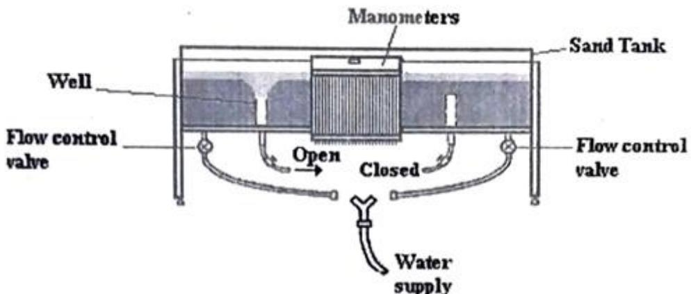
Groundwater abstraction from a well will result in the lowering of the water table and at the same time, a reduction of saturated depth available for the flow of water. The equation of flow for a constant discharge  $Q$  is given as follows.
